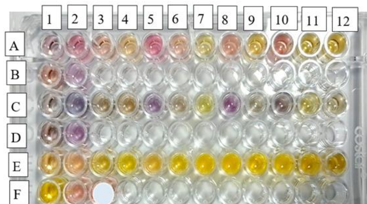
Figure 2. Color change of colloidal AuNPs synthesized using chili extracts of three varieties with different extract concentrations, pH and temperature. The sequence of images is described in table 1.
